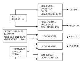
Fig: 9. Base modulation generator – HCBSVM
