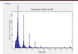
Fig: 14. FFT Plot DC Output Voltage and FFT Plot – HPSCPWM
