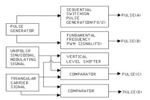
**Fig: 7.** Base modulation generator – HSCSPWM
