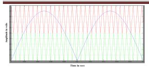
Fig: 2. Waveform pattern for APOD scheme
