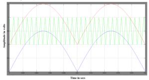
Fig: 3. Waveform pattern for SCSPWM scheme
