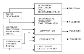
Fig: 6. Base modulation generator - HSCSPWM
